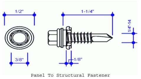
1/4-14 X 1-1/4" Carbon Steel Self Drilling Screw Type 3 Point - With Metal Backed Rubber Washer
