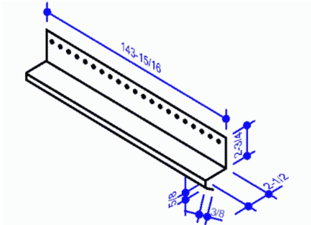
**BRII, Shadowall, or StylWall Base Trim at Flush, Notched, or Lapped Foundation**
